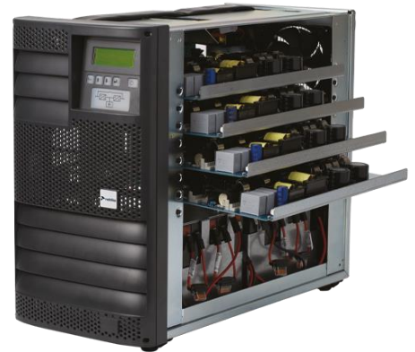
MINIPowerPLUS 10000 Fully populated with 8 Power Modules to offer a 10kVA system. Batteries are housed in a matching battery cabinet.
